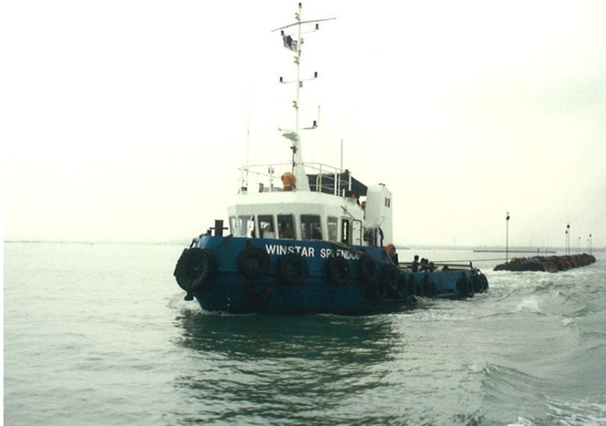
Towing of Floating Pipelines to Kepulauan Seribu using Winstar Splendour
